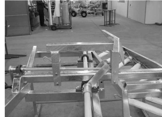
If required, bolt the tank bracket onto the spine making sure there is enough clearance for full travel of the suspension quadrants.
