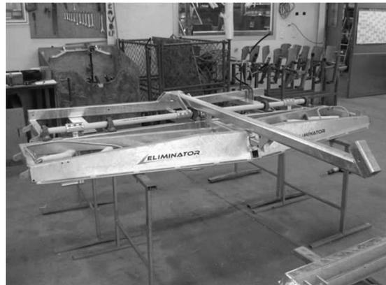
This part is a two man operation. Place the main frame and front carpeted frame onto trestles and clamp. Slide the spine onto the carpeted frame and main frame and bolt together.
