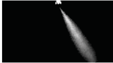
Inclined 30° spray pattern of medium to fine droplets provides superior coverage and canopy penetration.
