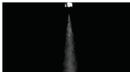
Dense spray pattern of smaller droplets to match many insecticide and fungicide applications.
